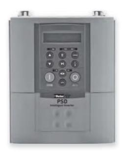
**PSD** AC variable speed drive has been designed to control the speed of refrigeration compressors. To improve system performance by matching compressor speed to cooling demand. The PSD has two dedicated analog inputs, 0 to 10 volts and 4-20mA, which can be used to control the speed of the compressor. The speed demand signals are provided by an external controller, such as Parker's **PSR** Rack Controller.
